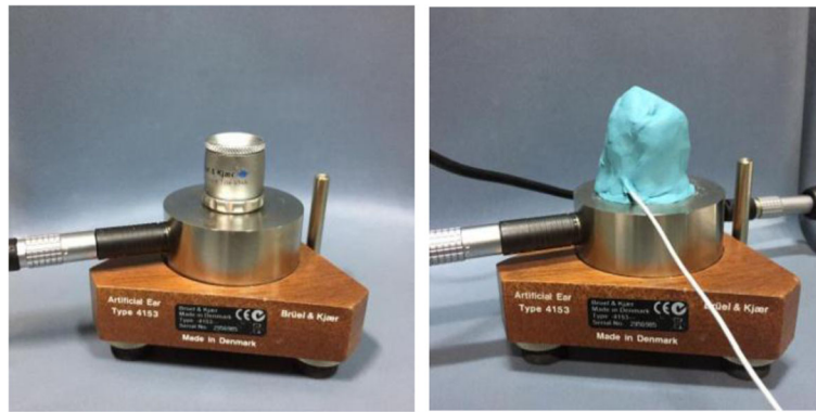
Fig. 1 Experimental design to measure sound pressure levels using the artificial ear and 2-cm 3 coupler (left panel) and earplug on the top of the measurement system (right panel)
