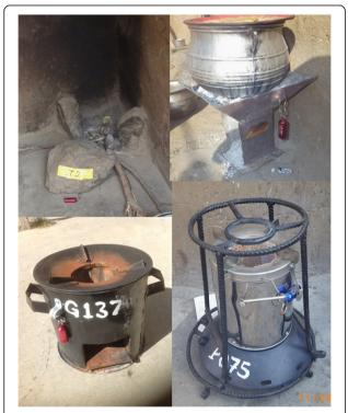
Figure 4 Traditional and improved stove technologies being compared in the REACCTING study, shown with Stove Use Monitors (SUMs) attached. Top left: traditional three-stone stove. Top right: traditional charcoal stove. Bottom left: Philips Smokeless Stove, Made in Lesotho (Southern Africa), Cost: ~US\$125. Bottom right: Gyapa Wood-Burning Stove. Made in Accra. Cost: ~US\$15-25.
