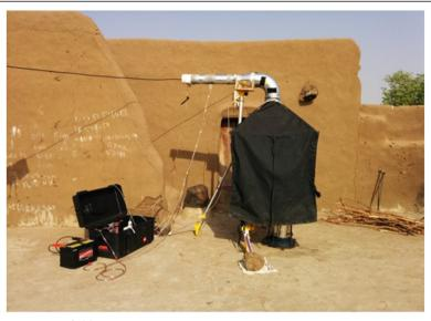
Figure 5 E-Pod setup for measuring in-field stove emissions.
